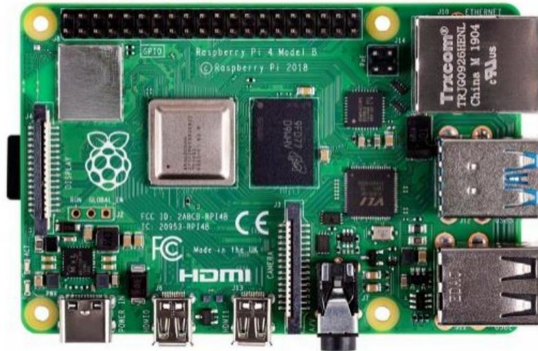
**Fig. 5: Raspberry Pi 4 modelo B.**
