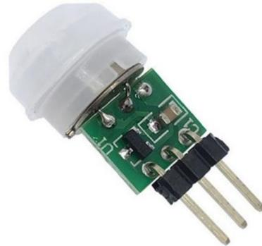
**Fig. 3. Sensor Mini PIR.**
